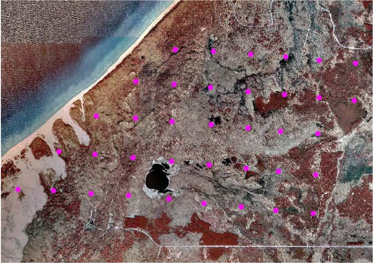
Figure 2. Point count sites were established 400 m apart in Mason County, Michigan, in a reference site established for a proposed wind energy development project. These sites were surveyed in April, May, June, September, October, and November 2007 for bird use.
